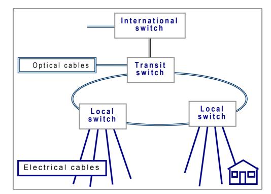
**Figure 4** – Switched Network: POTS network is depicted as an example of a switched network
